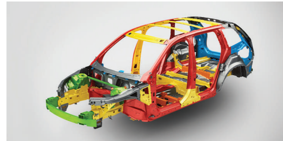
The body of the Volvo XC90 is designed for maximum strength around the passenger compartment and maximum energy dissipation in the front and rear crumple zones.
